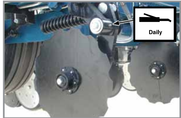
Notched single disc opener (1 per arm)
