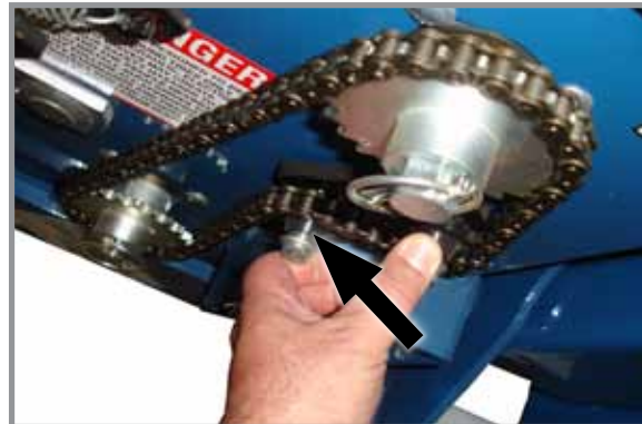
Chain idler tensioning
