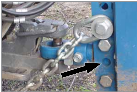
Clevis adjustment holes
