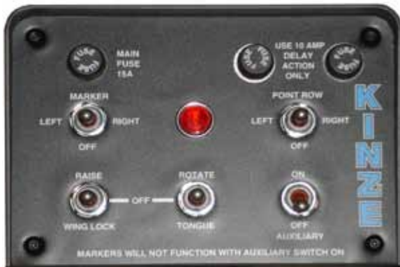
Single point row clutch control box
