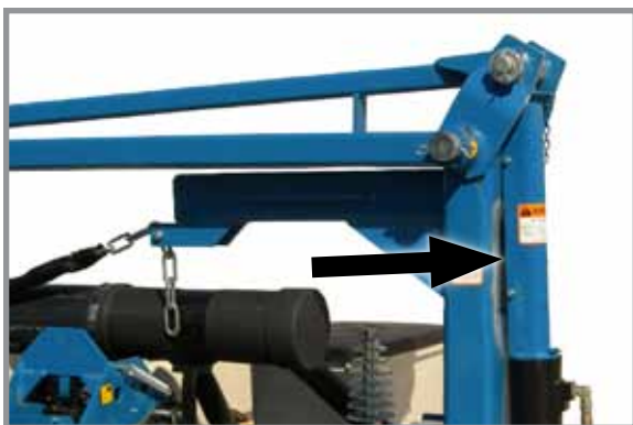
Row marker safety lockup installed
