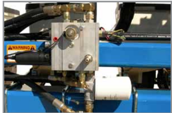
Vacuum fan valve block
