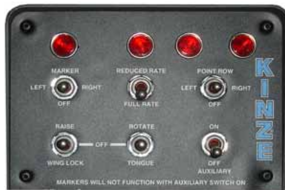
Two-speed point row clutch control box
