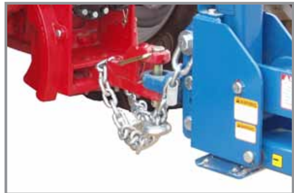
Tractor and safety chain hookup
