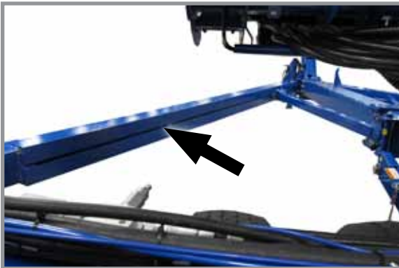
Axle link slide (L.H. shown)
