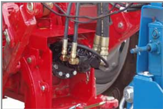
Two-section PTO hydraulic pump
