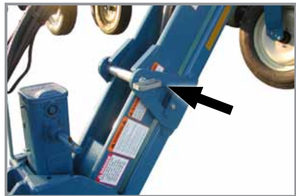
Hitch parallel linkage pin installed
