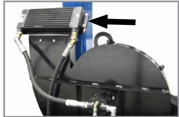
Oil cooler location
