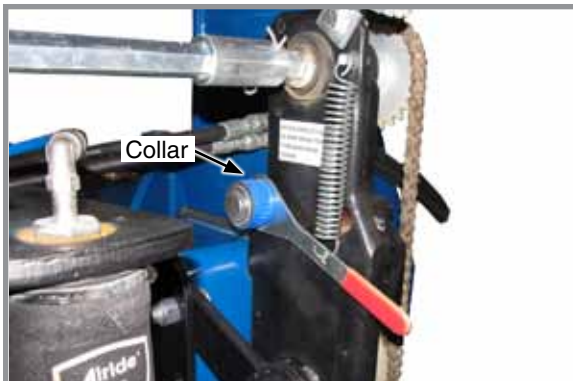
Wrap spring wrench (L.H. rotation shown)
