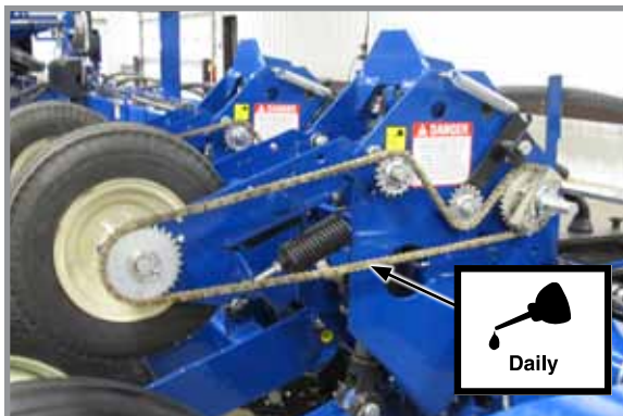
Contact wheel drive chains
