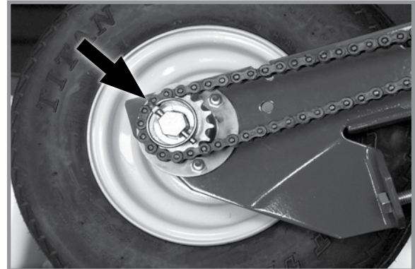
Optional half-rate drive sprocket
